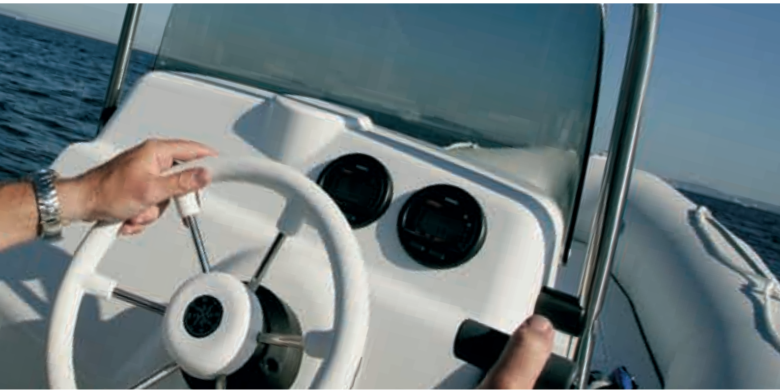
Diameter 350mm To fit this wheel, the special hub (YMM-24000-01-00) is required.
