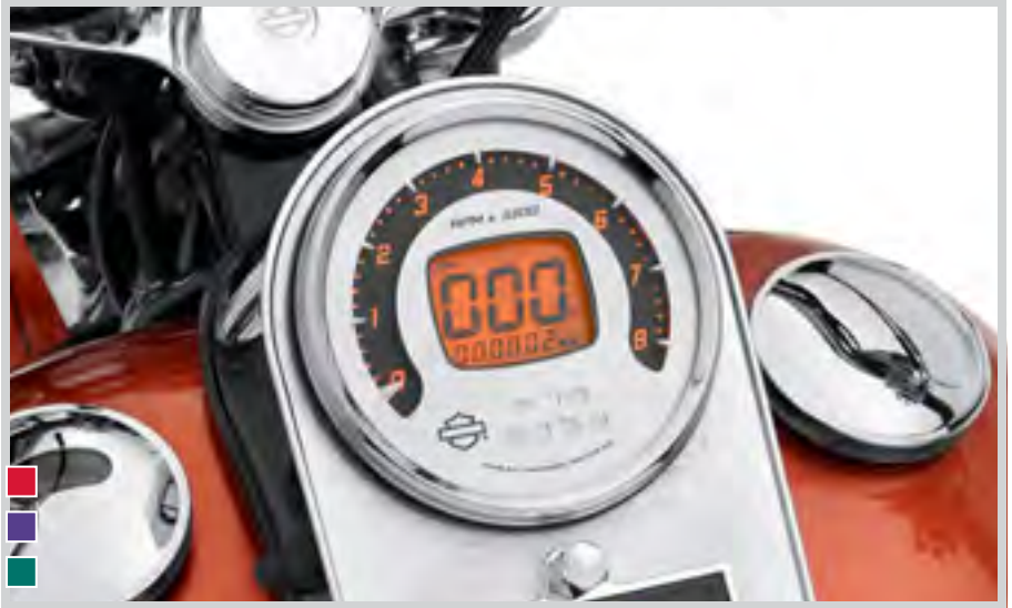
A. COMBINATION DIGITAL SPEEDOMETER/ANALOG TACHOMETER
