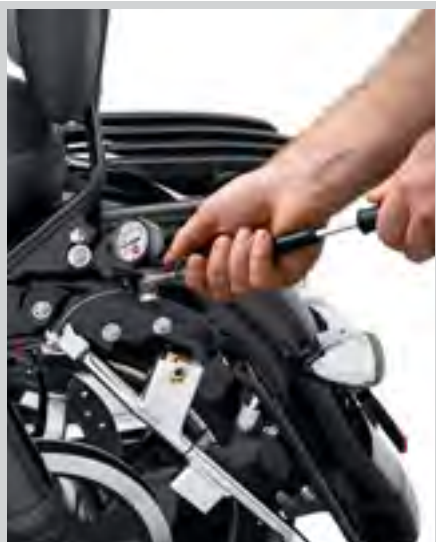
C. ANALOG TOURING SUSPENSION AIR PUMP
