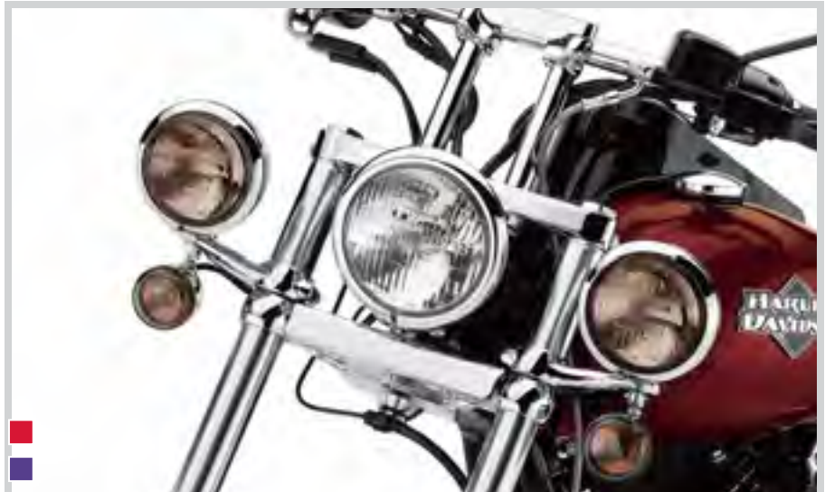
A. AUXILIARY LIGHTING KIT – FX SOFTAIL/DYNA WIDE GLIDE (SHOWN WITH AUXILIARY LAMP BULB KIT AND TURN SIGNAL RELOCATION KIT)
