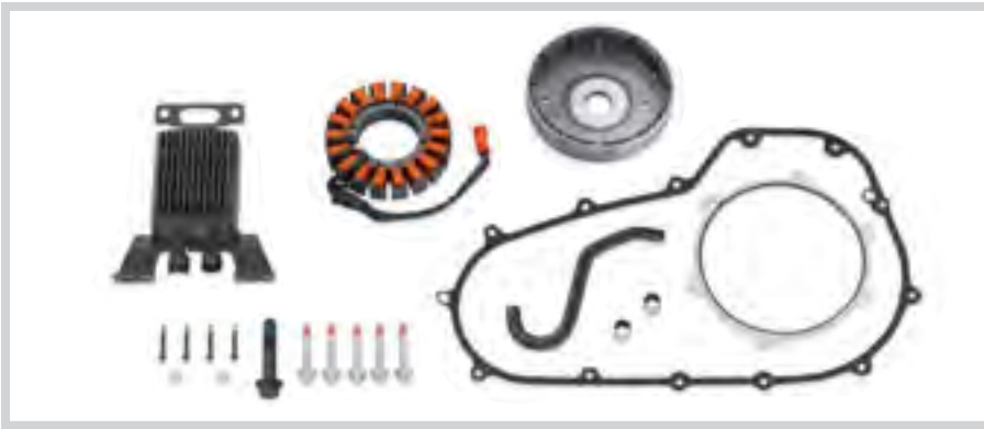
D. 54-AMP HIGH OUTPUT CHARGING SYSTEM
